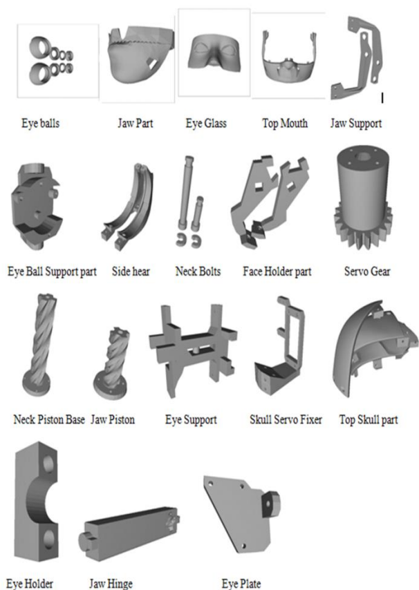
Fig 1: 3D printed parts of humanoid Robot
