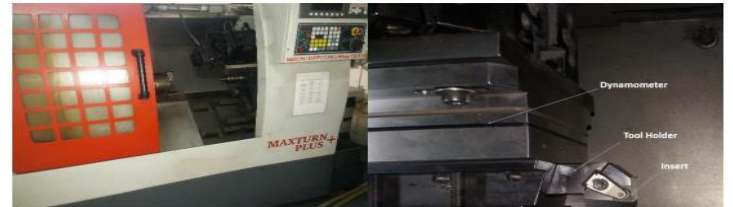
Fig. 3: Experimental setup on CNC machine
