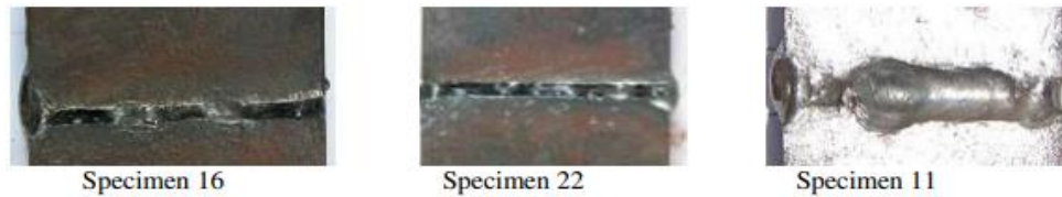
Fig. 4: Lack of penetration for experimental runs 16 and 22; sufficient penetration for specimen 11
