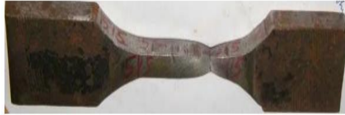
Fig.5: Specimen 21 after breaking in UTM
