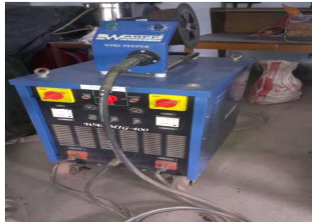
Fig.1: Flux cored arc welding
