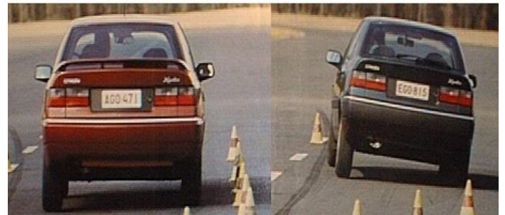
Figure 5: Cornering in a Xantia Activa and a normal Xantia [23].
