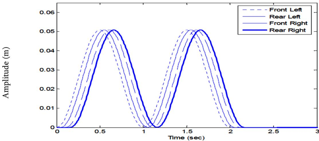
Figure 2: Bump road input disturbance for the front and rear wheels.
