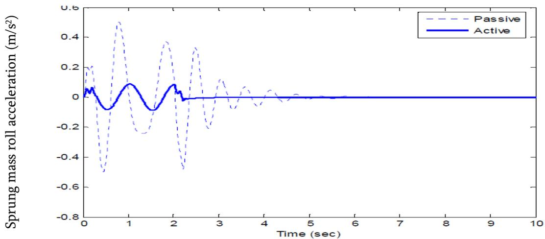
Figure 12: Sprung mass roll acceleration (m/s<sup>2</sup>)
