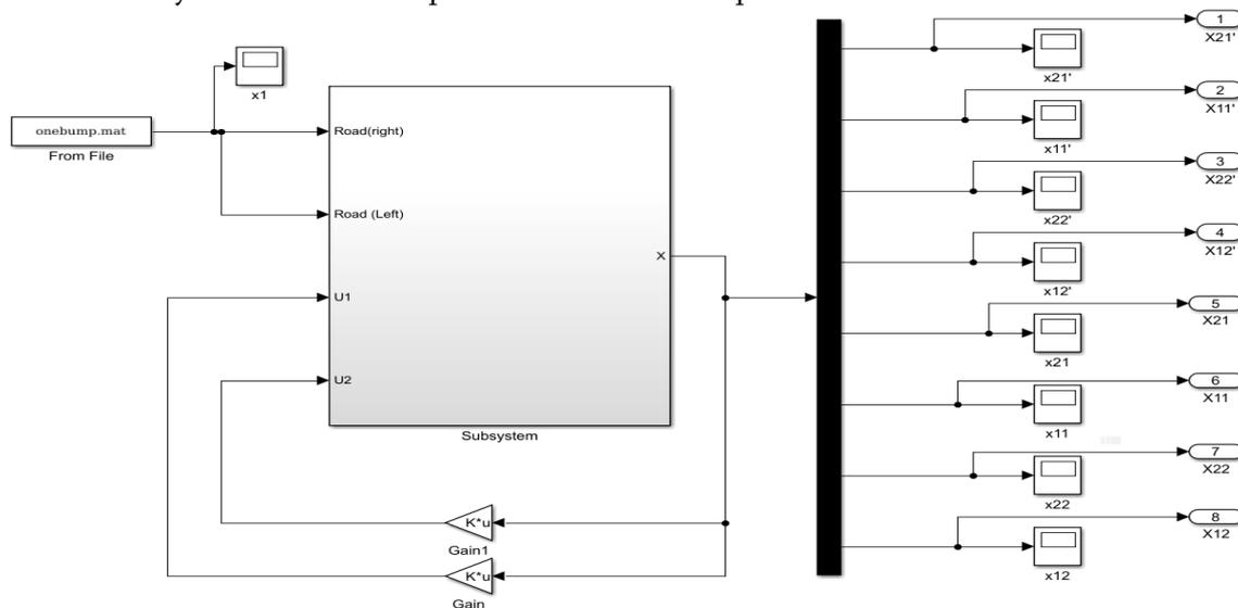
Figure 5. Half car 4 DOF passive suspension system
