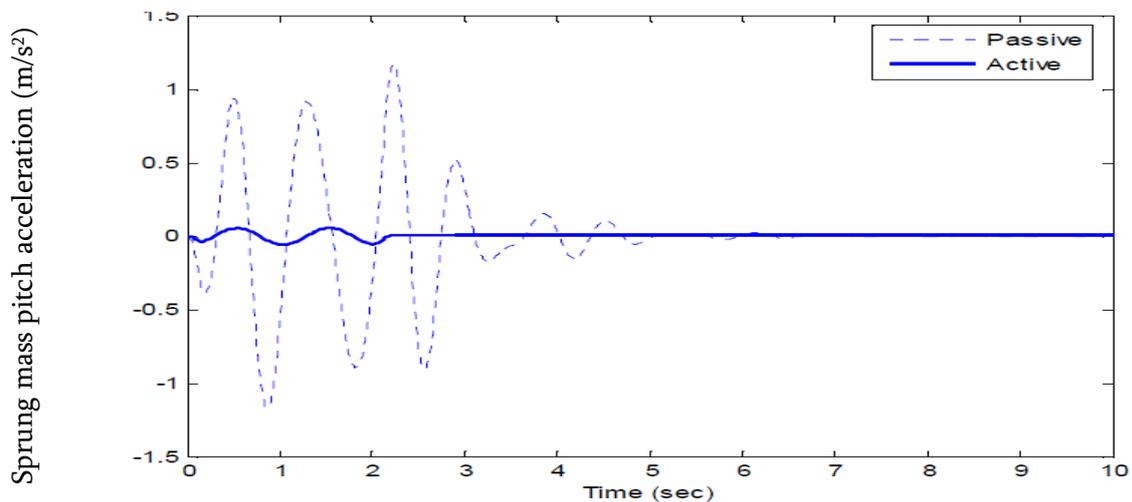
Figure. 13: Sprung mass pitch acceleration (m/s<sup>2</sup>)
