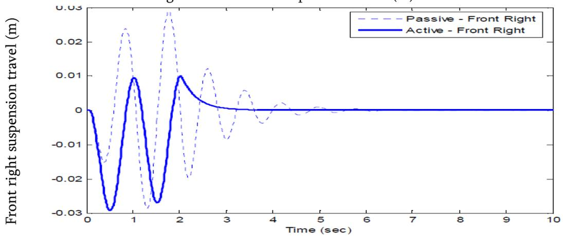
Figure 16: Front right suspension travel (m)
