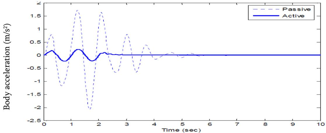
Figure 10: Vehicle body acceleration (m/s<sup>2</sup>)
