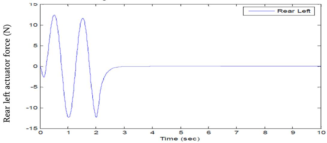
Figure 25: Rear left actuator force (F)
