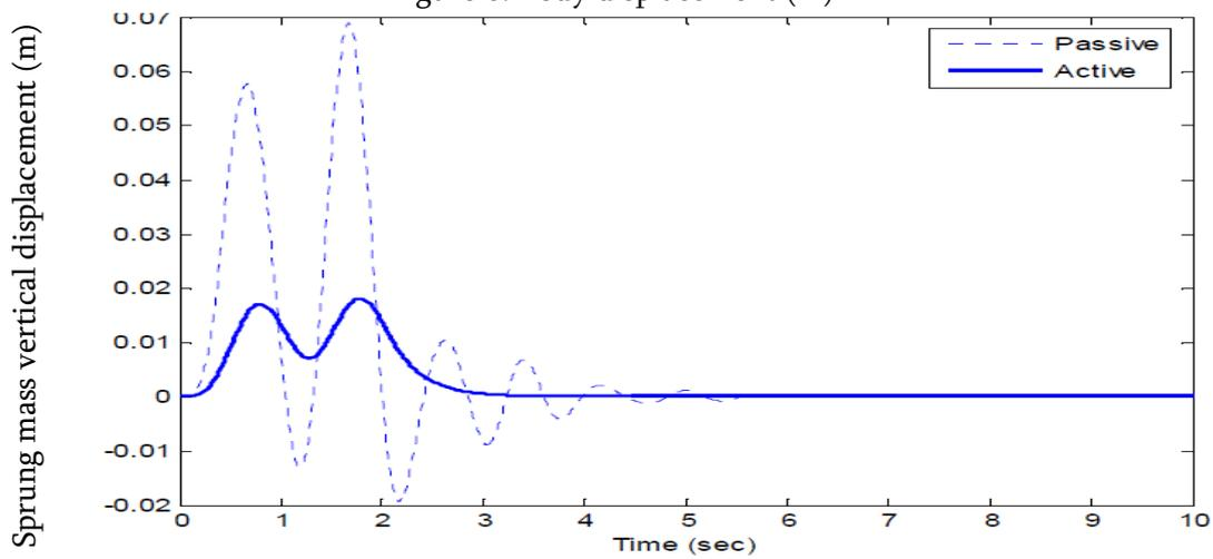
Figure 7: Vehicle sprung mass vertical displacement (m)
