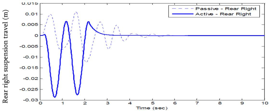
Figure 17: Rear right suspension travel (m)
