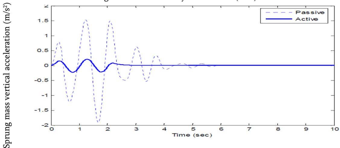
Figure 11: Sprung mass vertical acceleration (m/s<sup>2</sup>)
