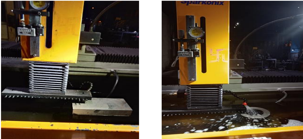
Fig.5: Machining process of Workpiece using EDM model 500 X Sparknix
