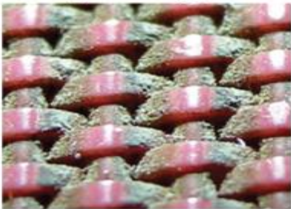
A plugged dirt stripe shown in an air permeability profile
