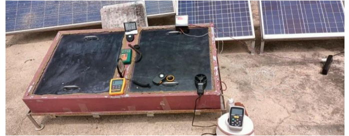
Fig.6: Solar distillation system
