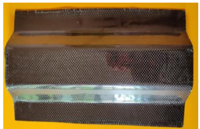
Figure 0-5 :Fabricated section after debulking
