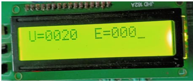
Fig 6. Distance of Object from user device (Car) using Ultrasonic Sensor
