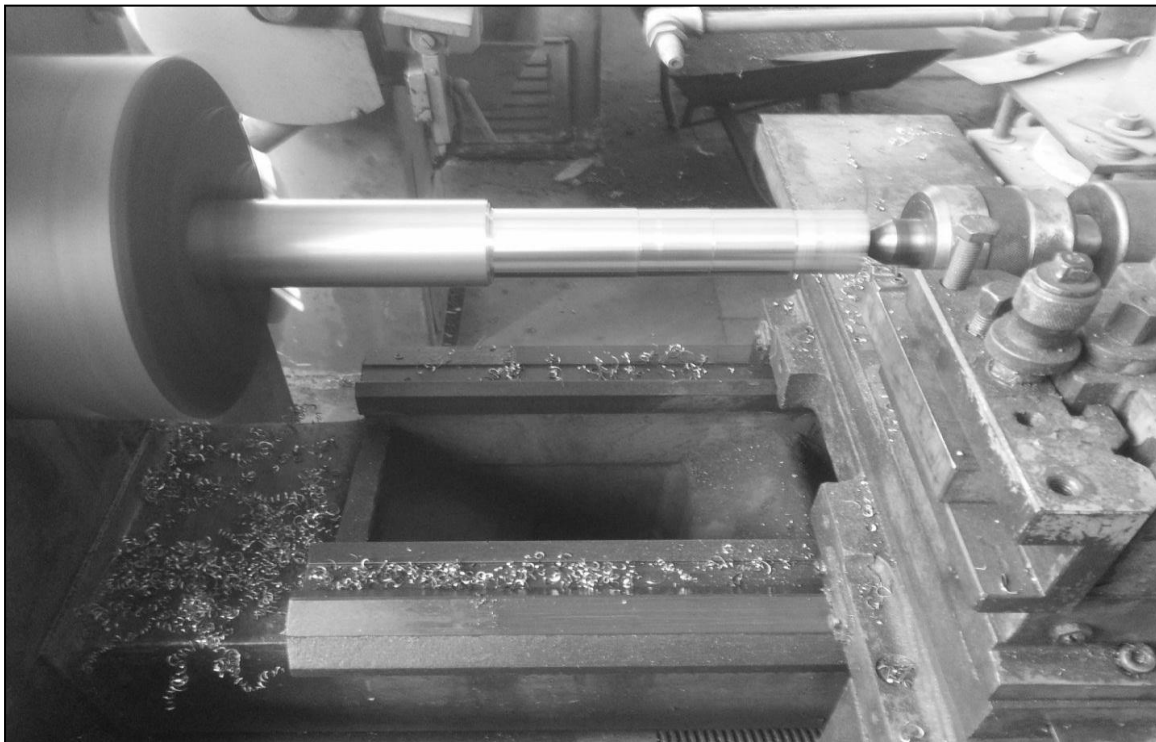
Fig 4: Mounting of tool and workpiece
