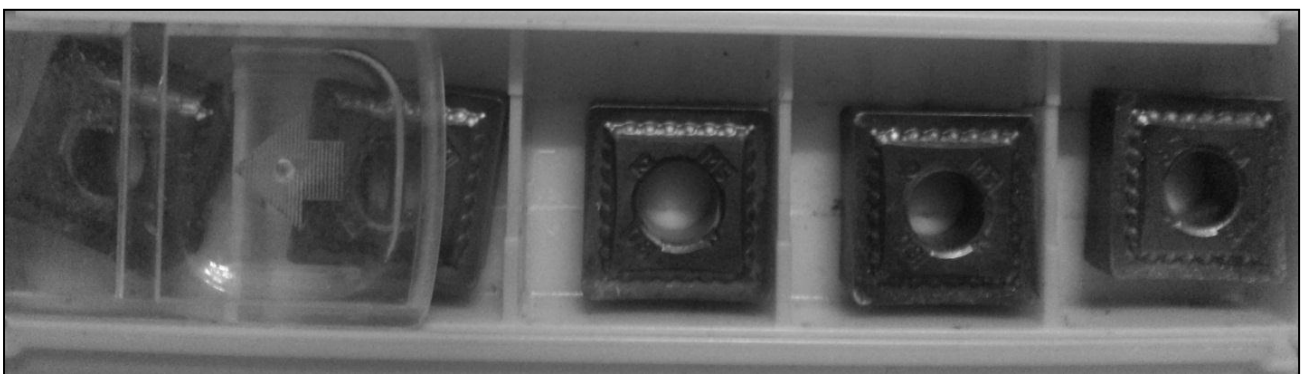
Fig 2: Set of cutting inserts used in the experimentation
