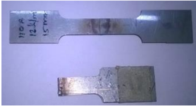
Fig.3. (b). Sample Tensile Test Specimen (Input parameters: C= 110 Amps, GF= 12, D= 15 mm)
