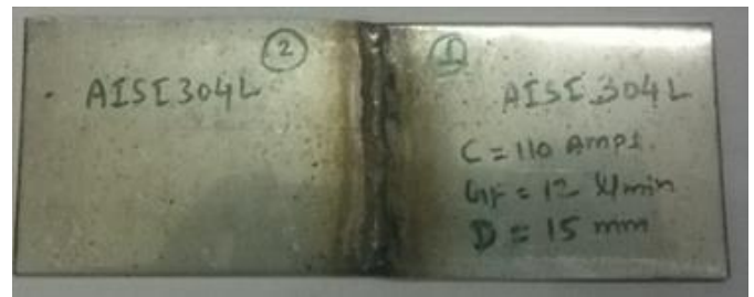
Fig. 2. TIG welded AISI 304L Specimen (Input parameters: C= 110 Amps, GF= 12, D= 15 mm)
