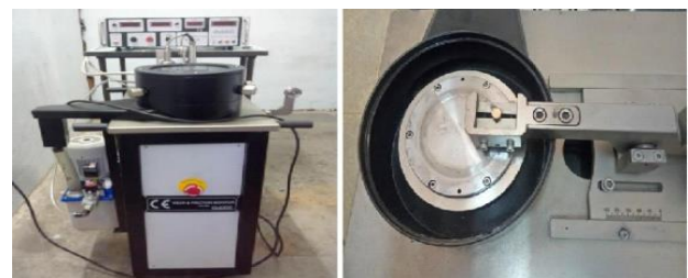
Figure 2.7 Pin on Disc Wear testing machine
