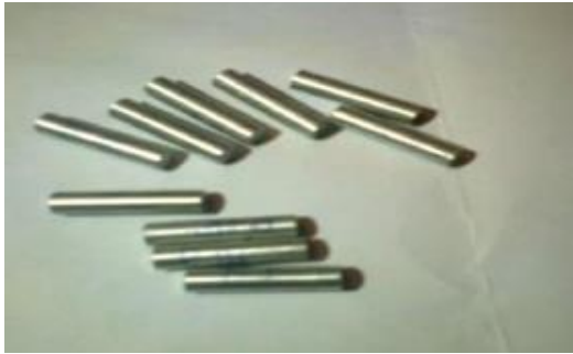
Figure 2.8 Machined specimen of wear test.
