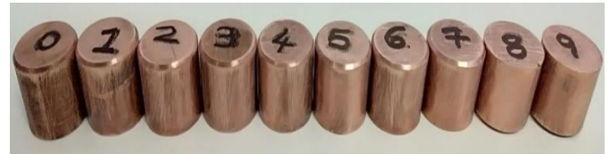
Figure 2.10 Corrosion test specimen before testing
