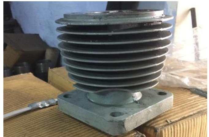
Fig.1.1 Air Compressor Fins mounted on cylinder block
