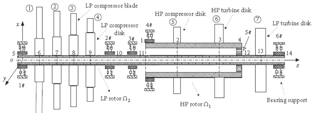
Figure 3. Dual rotor system model
