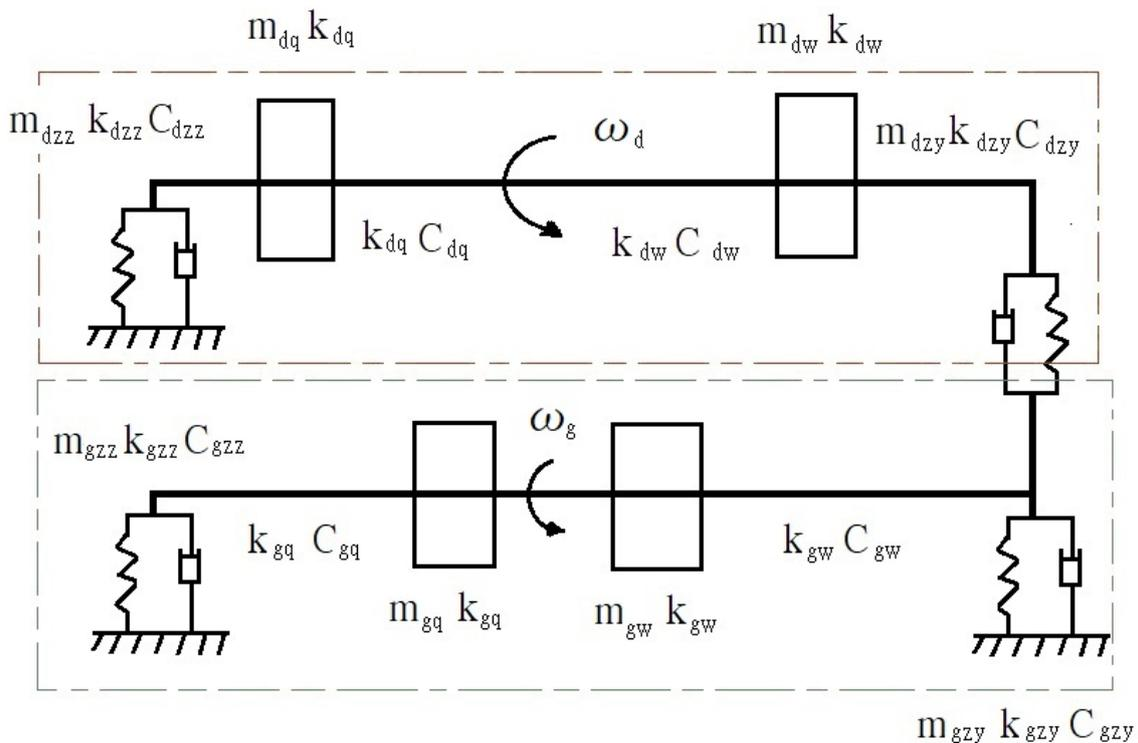
Figure 4. Mechanical model of dual rotor system
