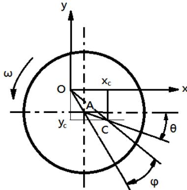
Figure 2. Rotor eccentric model
