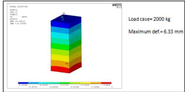
**Figure 14** Deformation of specimen load 2000 kg
