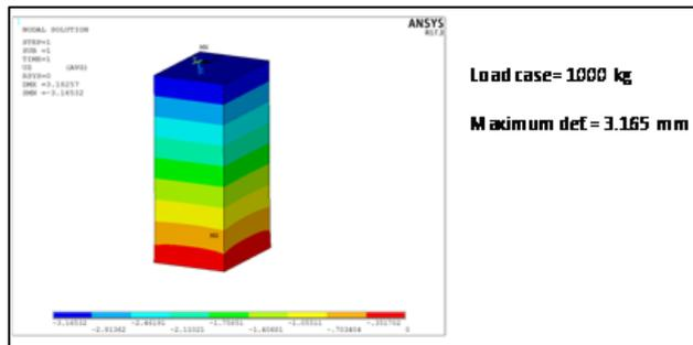
**Figure 13** Deformation of specimen load 1000 kg
