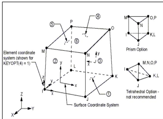
Figure 10 SOLID 45 Geometry
