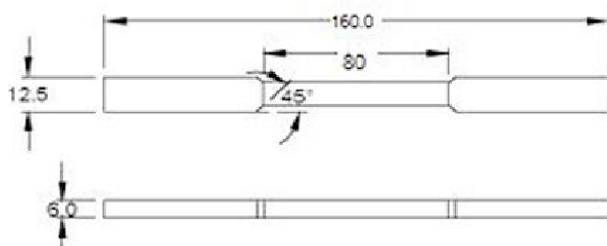
**Figure 3** Standard specimen for tensile test
