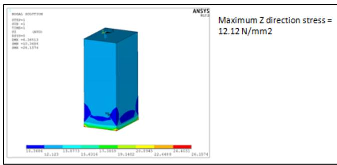
**Figure 17** Stresses in specimen load 2000 kg
