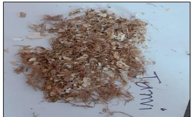
**Figure 1** Groundnut Shell and Coir Mixture
