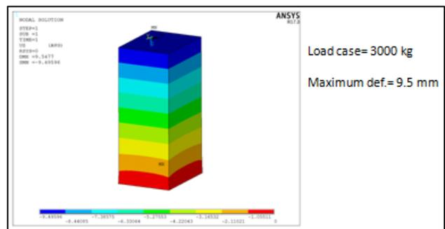
**Figure 15** Deformation of specimen load 3000 kg
