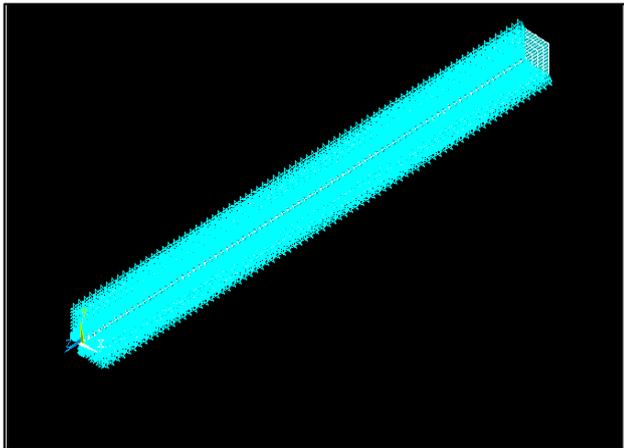
**Figure 12** Symmetric boundary conditions on quarter model
