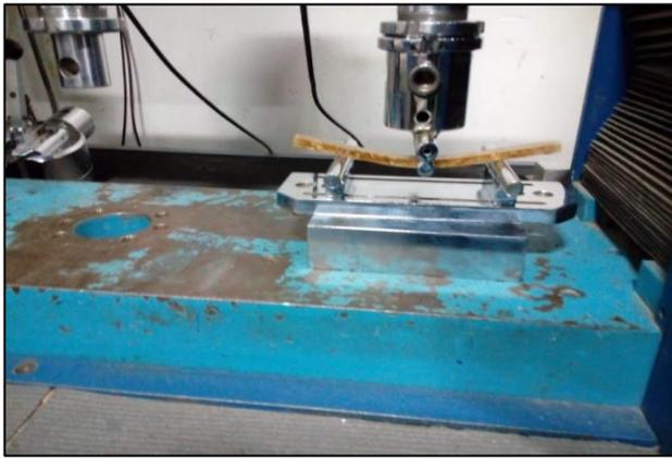
Figure 6 Flexural test setup
