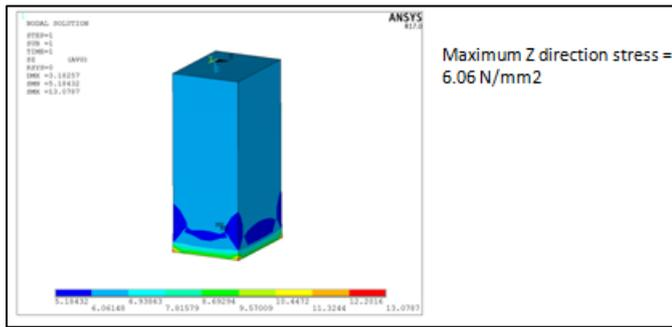
**Figure 16** Stresses in specimen load 1000 kg
