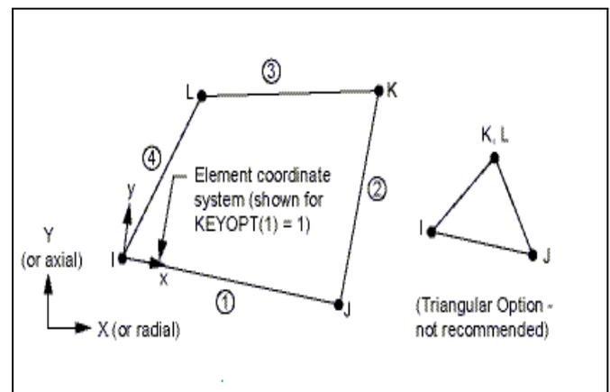
**Figure 8** PLANE42 Geometry
