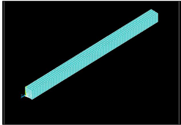
Figure 11 3D FE Model for Composite Specimen
