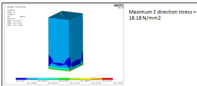
**Figure 18** Stresses in specimen load 3000 kg
