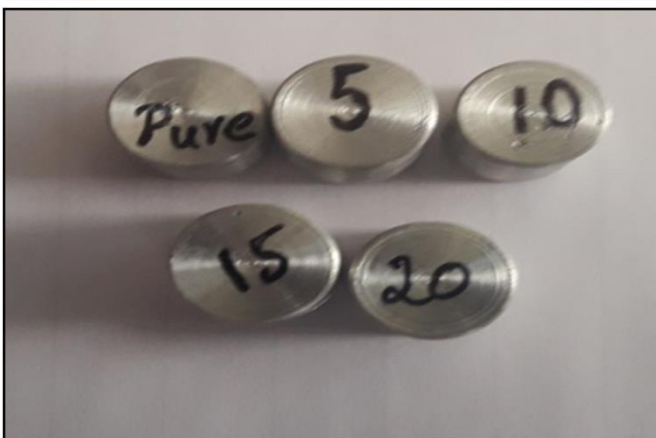
BHN test Samples
