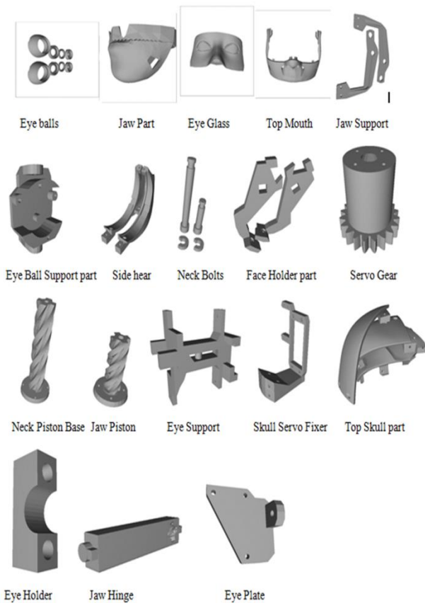
Fig 1: 3D printed parts of humanoid Robot
