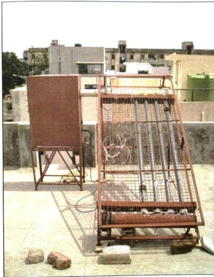
Fig.-1 Solar waste water evaporating system
