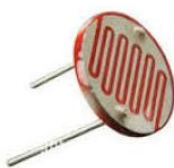
Fig. 1.4 : LDR – Light dependent resistor
