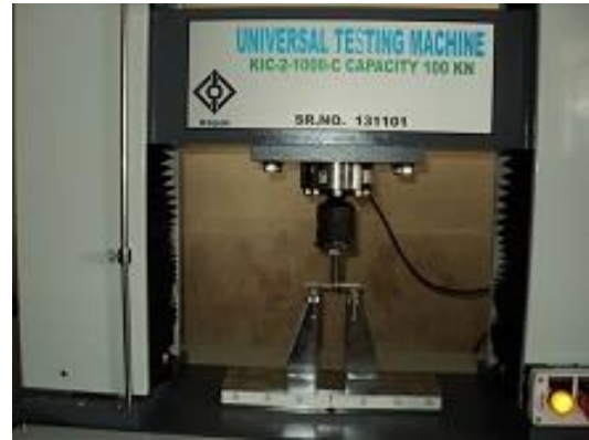
Fig 4. UTM MACHINE (three point bend test)
