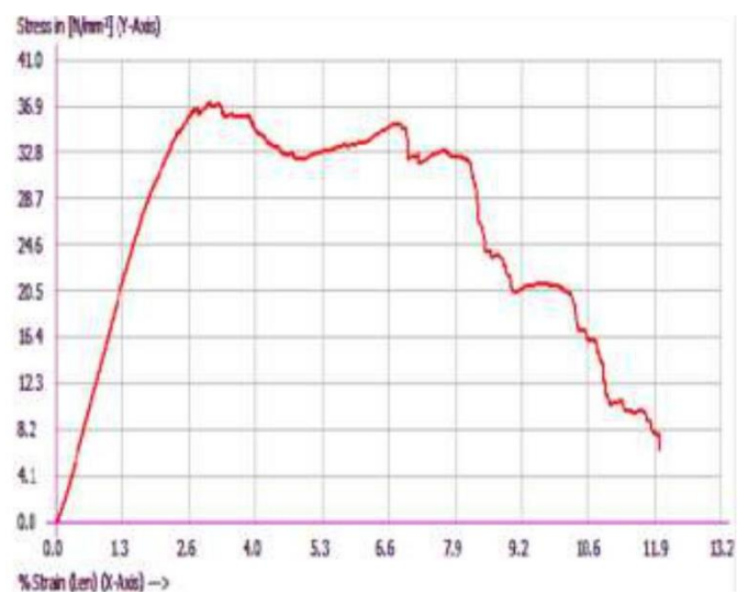
Figure 11. Stress v/s %strain for composite with 6% filler
