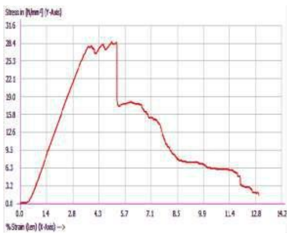
Figure 9. Stress v/s %strain for composite with 0% filler
