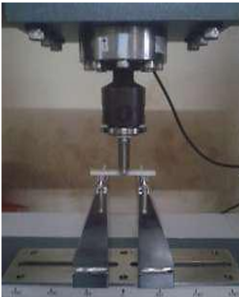
Figure 4 : - UTM setup for bending test
