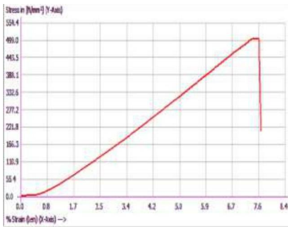
Figure 7. Stress v/s %strain for composite with 3% filler
