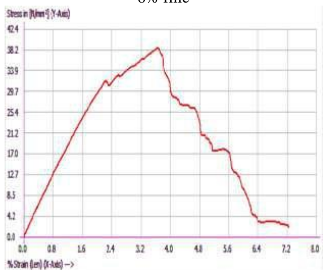
Figure 12. Stress v/s %strain for composite with 9% filler
