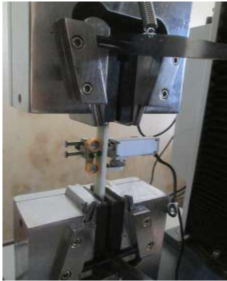
Figure 3 : - UTM setup for tensile test
