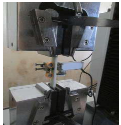
Fig 4: UTM machine (for tensile test)
