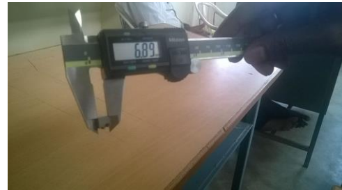
Figure 7. Measurement of width in vernier calipers
