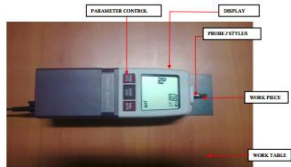
Figure 8. Mitutoyo surftest SJ-201P instrument
