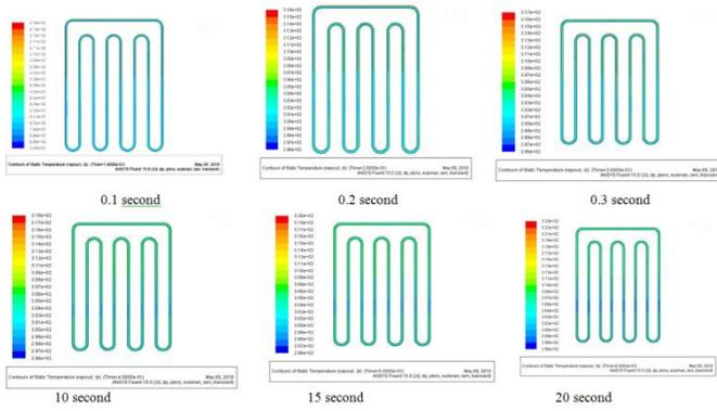
**Figure 6.** Temperature distribution in the Heat pipe
