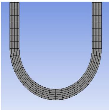
**Figure 3** Shows the Meshing configuration of 2D CLPHP used in simulation.
