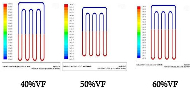
**Figure 4** Different filling ratio of FC-72 in CLPHP
