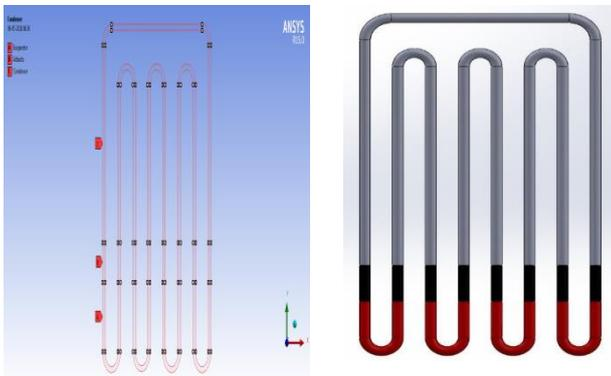
**Figure 2.** Physical model of Closed loop pulsating Heat pipe
