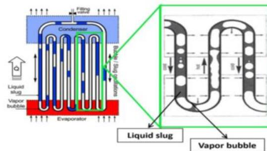
**Figure 1.** Basic scheme of a closed loop PHP, on the right, zoom of the internal flow patterns.
