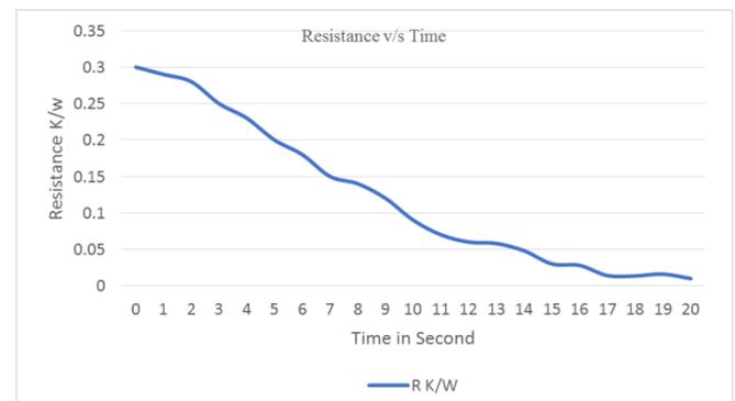
**Figure 8.** Graph plotted thermal resistance v/s Time
