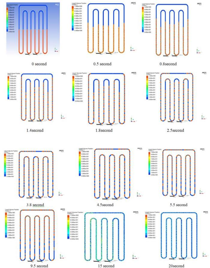
**Figure 5.** Flow visualization of the PHP and Liquid slugs ,vapour bubbles in the tube
