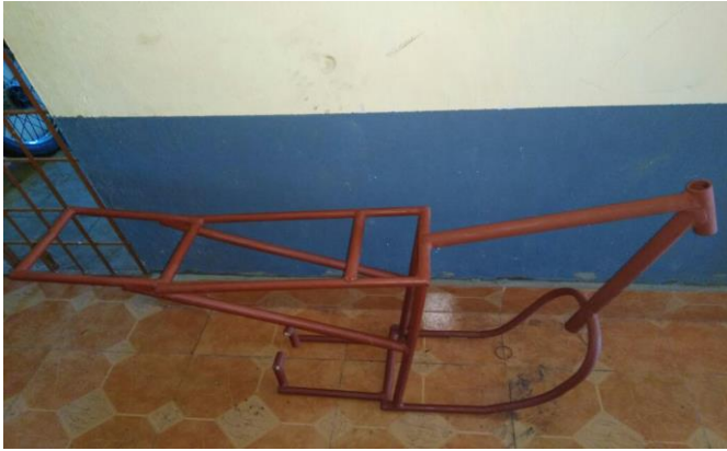
Figure 3.1. Fabrication of motorcycle frame
