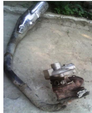
Figure 1.3. Turbocharger Connection with Bike Silencer
