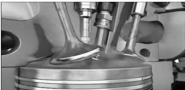
Figure 1.2. GDI Function Inside Combustion Chamber.
