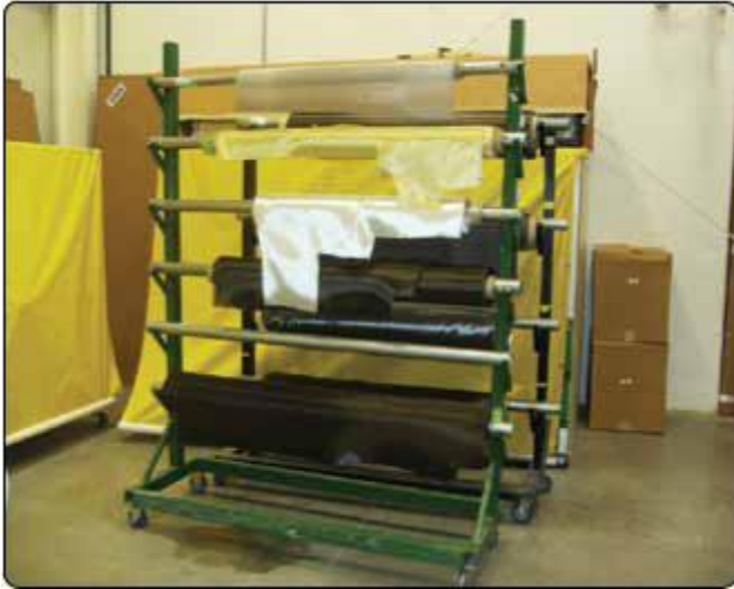
Figure 12. Dry fabric materials (top to bottom: aluminum lightning protection mess, Kevlar, fiberglass, and carbon fiber).
