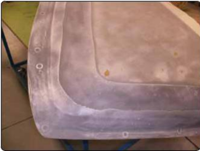
Figure 9. Aluminum meshes lightning protection material.
