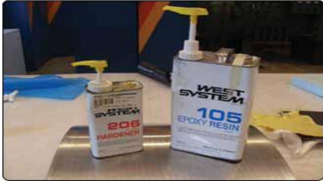
Figure 10. Two part wet layup epoxy resin system with pump dispenser.
