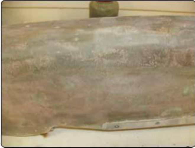
Figure 8. Aluminum meshes lightning protection material.
