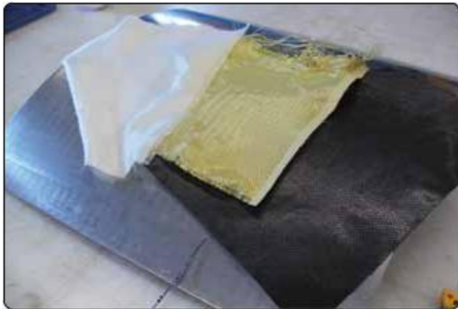
Figure 7. Fiberglass (left), Kevlar (middle), and carbon fiber material (right).
