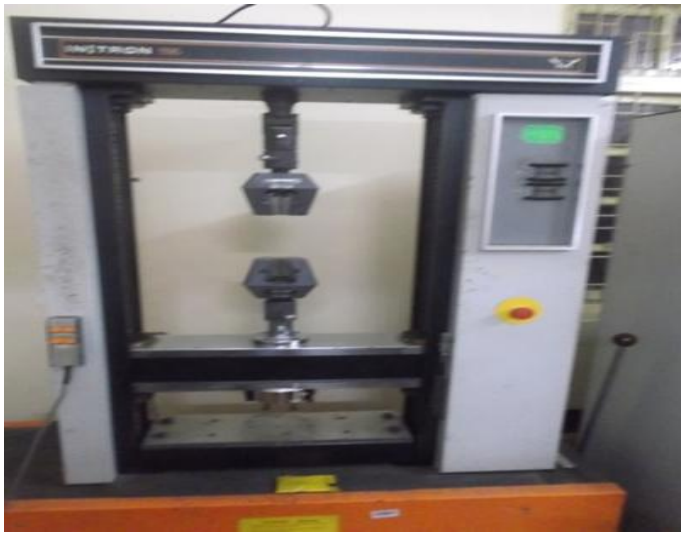
Figure 3. Experimental set up for tensile test with universal testing machine, Instron 1195
